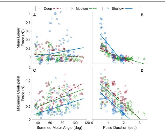
**Figure 7.** Linear models between measured motor kinematics and whole-body forces in the three robotic models. Panes (A) and (B) show the relationships between the measured control variables and linear forces. Panes (C) and (D) show the relationships between the measured motor control variables and centripetal forces. These forces are estimates based on the volume of each model, as discussed in the methods section.
