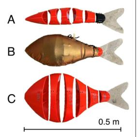
**Figure 2.** Body shells for each robot shape: (A) shallow, (B) medium, (C) deep. The medium shape shows the fully assembled robot with tailored skin.
