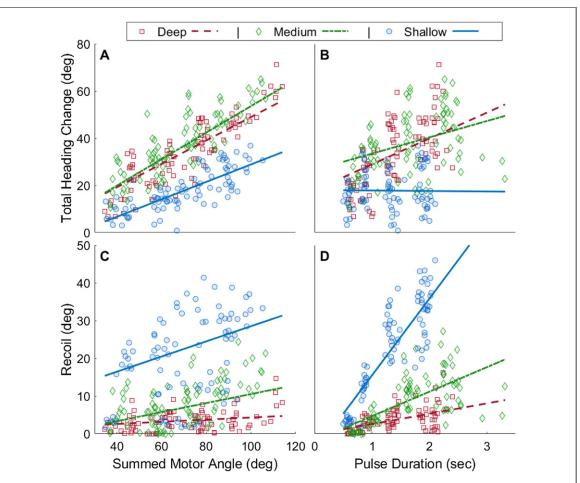
**Figure 5.** Linear models between measured motor kinematics and heading change variables in the three robotic models. Panes (A) and (B) show the relationships between the measured control variables and total heading change. Panes (C) and (D) show the relationships between the measured motor control variables and recoil.
