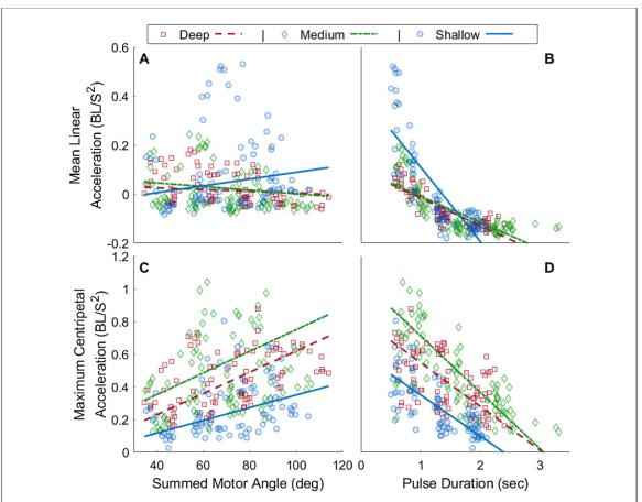
**Figure 6.** Linear models between measured motor kinematics and whole-body accelerations in the three robotic models. Panes (A) and (B) show the relationships between the measured control variables and linear acceleration. Panes (C) and (D) show the relationships between the measured motor control variables and centripetal acceleration.
