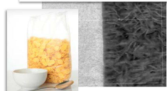
Epitaxial lamellae at barrier-tie interface: heat sealed food packaging
