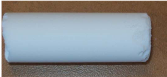
Figure 2. POSS-reinforced aerogel cylinders with 3 times higher compressive modulus compared to tetraethoxy silane-based aerogels
